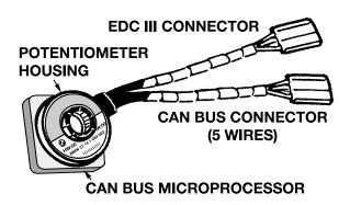
The sensor still utilizes two potentiometers to determine the steering angle and the rate of steering. These are the raw signals the CAN Bus microprocessor utilizes to create the steering angle signal for broadcast on the CAN bus.
